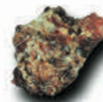
Granite Igneous; formed when molten rock cools underground
